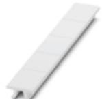
Zack marker strip, Strip, white, unlabeled, can be labeled with: PLOTMARK, CMS-P1-PLOTTER, mounting type: snap into tall marker groove, for terminal block width: 15.2 mm, lettering field size: 10.5 x 15.1 mm, Number of individual labels: 5
