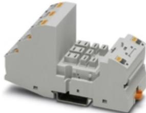
Relay base RIF-4..., for high-power relay with 2 or 3 changeover contacts or 3 N/O contacts, Push-in connection, plug-in option for input/interference suppression modules, for mounting on NS 35/7,5
