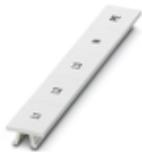
Zack marker strip, Strip, white, labeled, printed horizontally: L1, L2, L3, N, PE, mounting type: snap into tall marker groove, for terminal block width: 15.2 mm, lettering field size: 10.5 x 15.1 mm, Number of individual labels: 5
